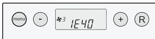
Blokkerende storing; ventilator storing
