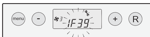
Vergrendelende storing; ventilator storing Storingsweergave knippert
