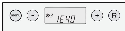
Blokkerende storing; ventilator storing
