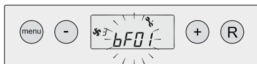
Vergrendelende storing; ventilator storing Storingsweergave knippert
