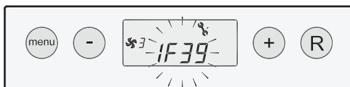
Vergrendelende storing; ventilator storing Storingsweergave knippert
