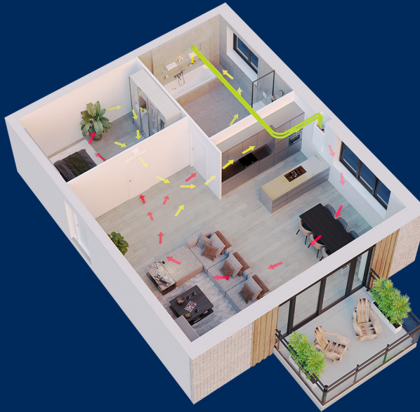
Two-room apartment with Ease 100 as semi-central ventilation (recessed) with an extra indoor mixfan between the living room and bedroom.
