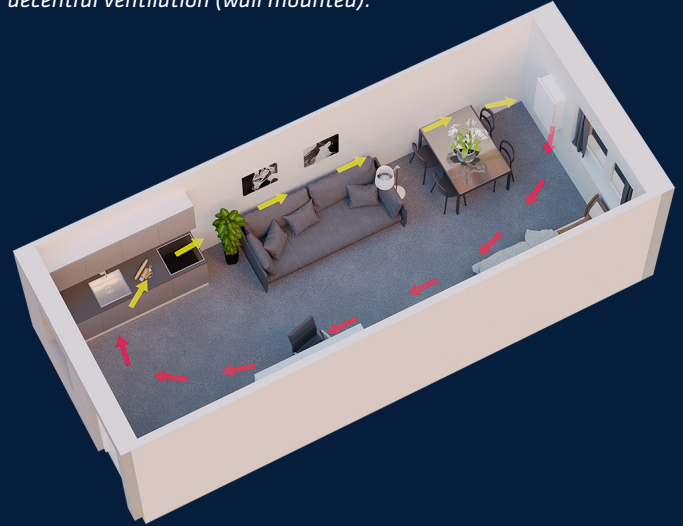
Student accommodation or assisted living facility with Ease 100 as decentral ventilation (wall mounted).
