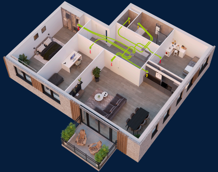
Ease 200 installed in a kitchen cupboard in an apartment.
