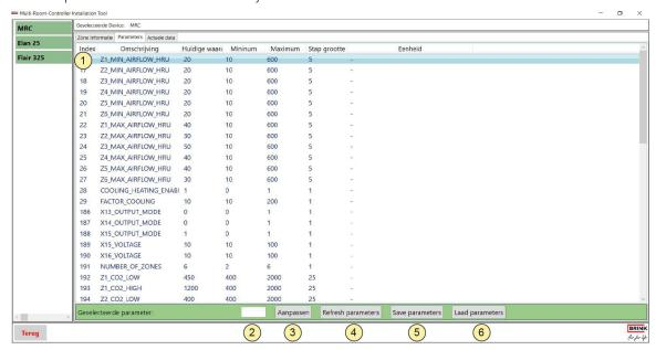
Follow the steps below to save the complete configuration of a Multi Room Controller system for reuse or to load complete configurations into other Multi Room Controller systems. This can be useful when replacing the Multi Room Controller board or in projects where several of the same systems are installed.
